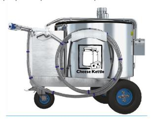
At the stages of heating, pasteurization and cooling both parts (panel supply and mobile tank on wheels) are connected with each other using the power cable and two high pressure hoses of hot/cold water supply.
